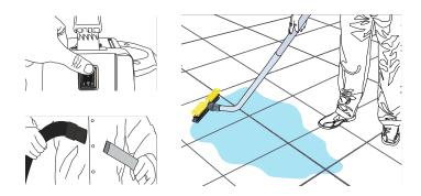
Vacuum floor surface diagonally to grout lines, reaching under shelves, seating etc.
