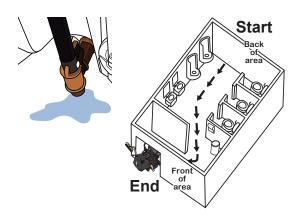
Turn Vacuum Motor to ON. Attach Vacuum Wand to Vacuum Hose (if not already connected).
