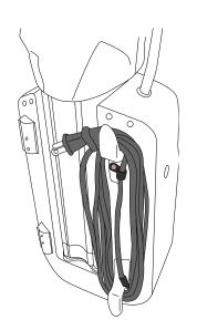
To charge the battery, keep the battery in the battery housing. Locate the cord wrapped around the cleats connected to the battery housing, plug into an outlet to begin charging.
