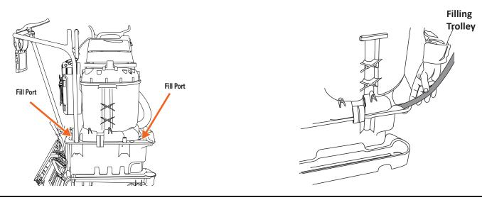
Note the location of the Fill Marker inside the Trolley Bucket.
