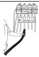
Rinse Vacuum Tank thoroughly at clean-up sink, preferably with hot water. Rinse out Trolley Bucket. Rinse foam filter inside Vacuum Tank and Trolley Bucket. Rinse plastic finger filter in both components following to clear debris. Clean the mixing solution assembly and orifice.
